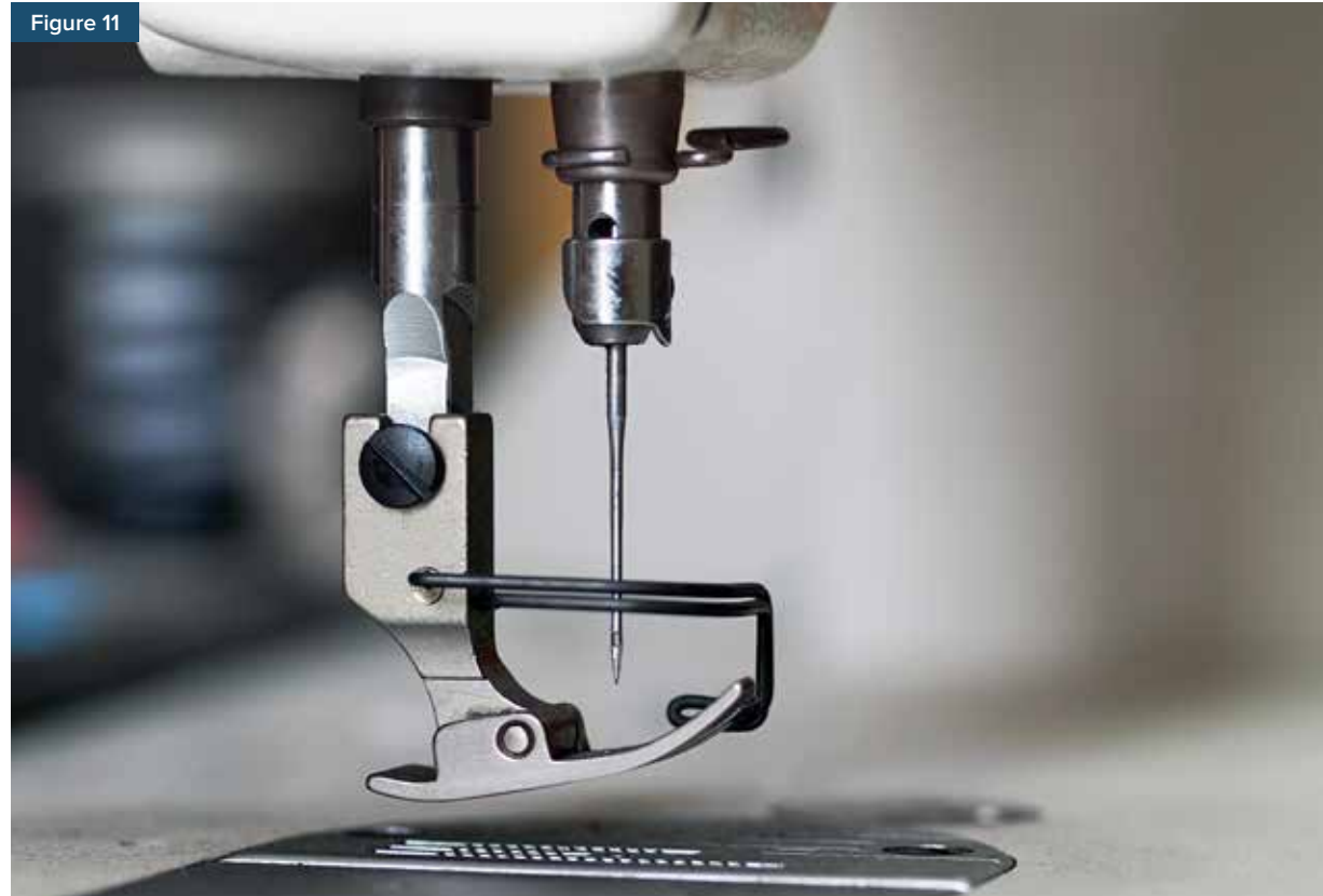
Proper needle guarding on a sewing machine
