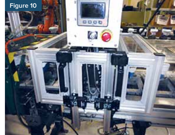
Machine enclosure preventing contact with moving parts
