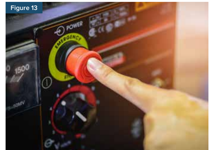
Machine with emergency stop switch
